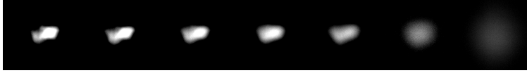
Figure (4.8) Free expansion of a cold atomic cloud viewed with a camera with a certain delay: 0, 100 \mu s, 500 \mu s, 750 \mu s, 1000 \mu s, 2000 \mu s, 3500 \mu s.
